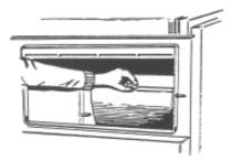
The firebox ceiling has an angled rib which has a step in its height. This angled rib goes on top and toward the front of the firebox. Again this casting rests on top of the ledges. Lift one end over the ledge at a time as before. When finally in position, its rear edge tucks under the 'joggle' along the front edge of the rear upper wall casting.
