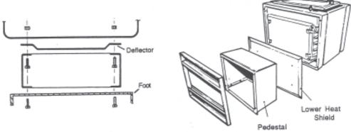
If your woodfire has pedestal trims, these are to be clamped between the pedestal and the pedestal foot. the simplest way to do this is to hold the trims in position with sticky tape before fitting the foot using the four screws provided. Position the trims accurately before fully tightening the screws.
