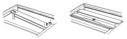
The Cashmere is supplied with four fire bricks. Two bricks fit across the back with their chamfered comers positioned to clear the tie rods in the comers of the firebox, and one brick fits each side with its chamfered comer facing the door opening.
