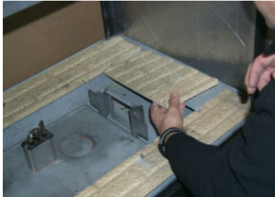
Remove Left & Right Side Base Brick Panels
